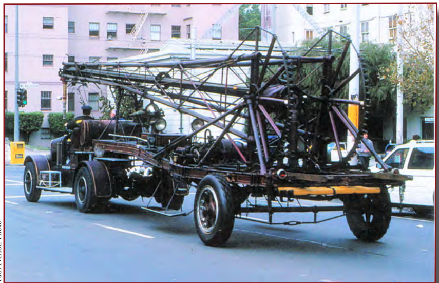
SFFD Water Tower 1926 Klieber tractor, 1902 Gorter tower, 75-ft
