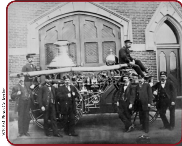
Engine M 1863 Silsby 400gpm rotary pump
