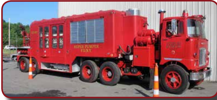
1965 Former FDNY Super Pumper; one of 6-units Designed by Gibbs & Cox naval architects Mack 715FST Highway Tractor 2400hp Napier Deltic engine; 6-stage, 8800gpm DeLaval pump
