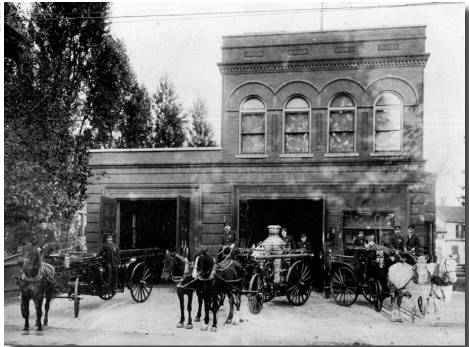
Glenville Firehouse, CFD Station No. 30, Built 1898. Glenville apparatus acquired and used by Cleveland (left) village ladder truck manned by E30 when needed (center) 1904 American steamer 4 th size, double piston, 450gpm (right) hose wagon for steamer
