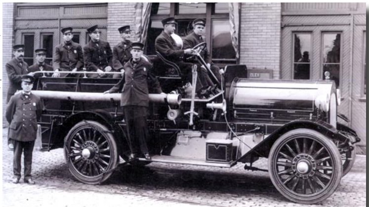
1917 Type 12 ALF, 750gpm rotary pump as Engine Co. 39
