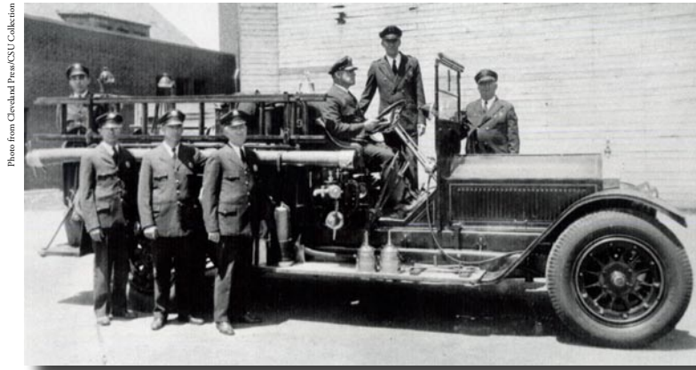
1912 Nott, 600gpm rotary gear pumper as Engine Co. 34
