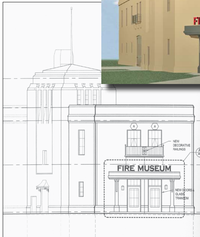
Doty and Miller Architects have developed this design for what will be the new entrance to the Fire Museum. Instead of cutting a new opening in the side of the historic facade, this design makes use of the original windows at the east end of the building and converts them into the new doors. The new entrance is clearly marked by the Fire Museum sign above the portico.
