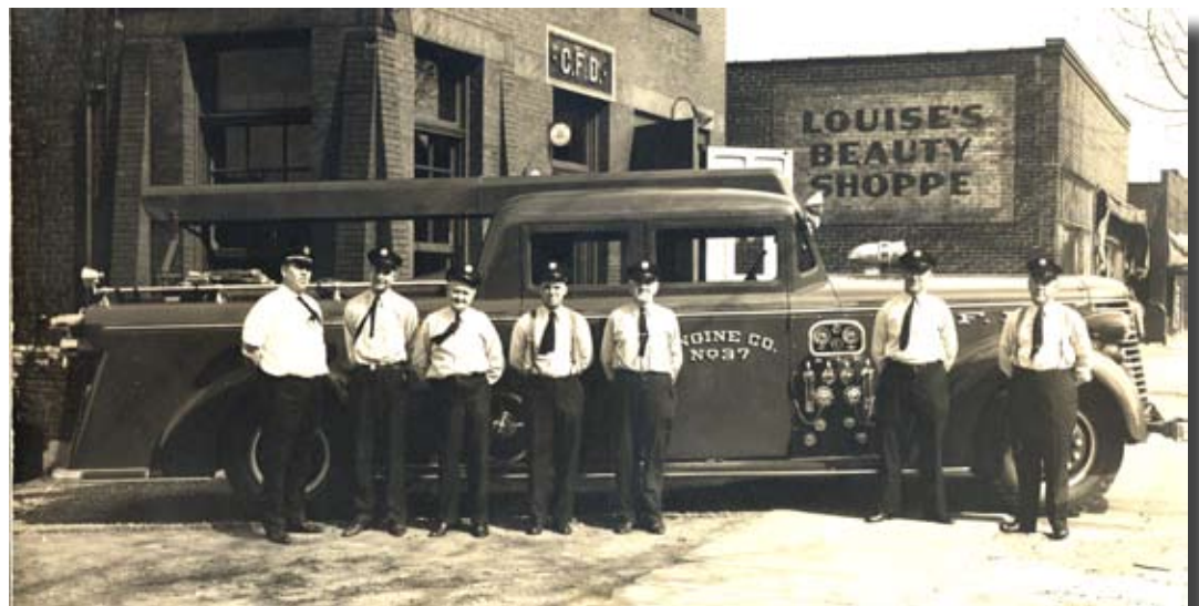
1939 American LaFrance (500 Series), 1000 gpm (31F7) and crew in front of station at 2314 Broadview Avenue, SE (WRFMC Collection)
