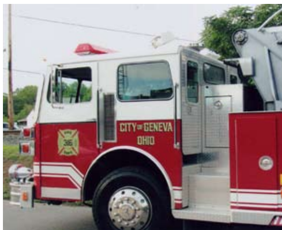
Geneva 1983, Sutphen 1500/500/65-ft, Rehab by Precision. Two ex-Cleveland rigs are in service in Ashtabula County, both 1983 Sutphen mini towers that have been rehabbed to like-new condition. They look quite similar to the days of their service in the City with the exception of doors added to enclose the jump seats. The refurbished rigs are located in Geneva and Trumbull Township but it is not clear where they were used in Cleveland.
