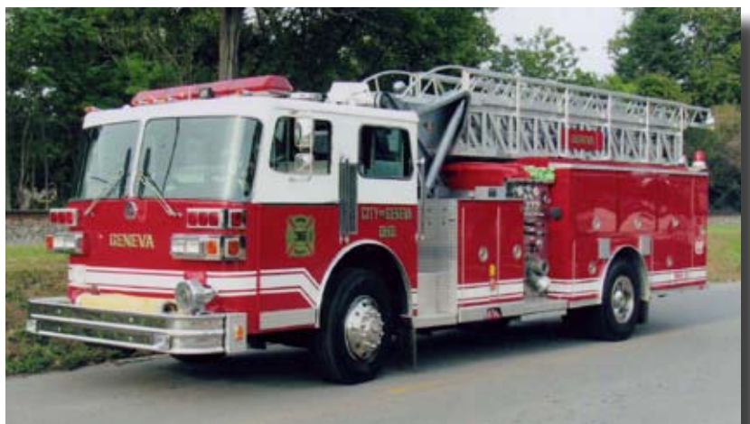
Geneva 1983, Sutphen 1500/500/65-ft, Rehab by Precision. Two ex-Cleveland rigs are in service in Ashtabula County, both 1983 Sutphen mini towers that have been rehabbed to like-new condition. They look quite similar to the days of their service in the City with the exception of doors added to enclose the jump seats. The refurbished rigs are located in Geneva and Trumbull Township but it is not clear where they were used in Cleveland.
