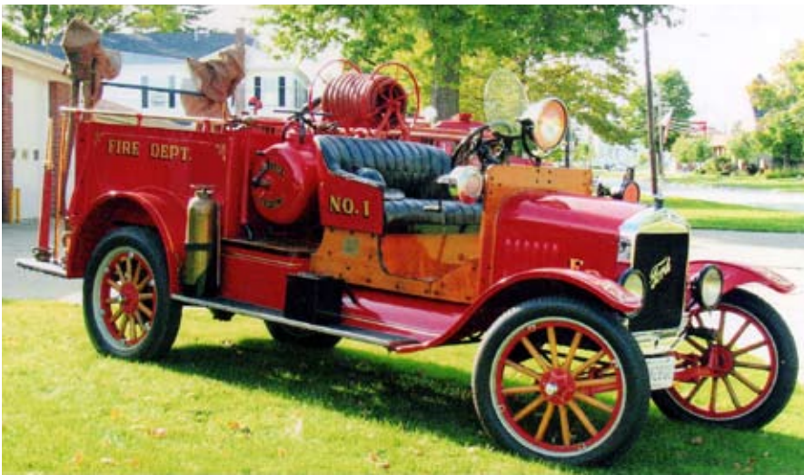
Jefferson 1924 Prospect/Model T Chemical engine. Originally from the Sugar Creek area. Note the two Garret Morgan smoke masks at the rear
