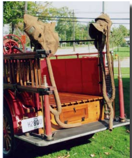
Jefferson 1924 Prospect/Model T Chemical engine. Originally from the Sugar Creek area. Note the two Garret Morgan smoke masks at the rear
