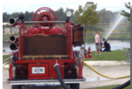
SEAGRAVE PUMPS 2 LINES FROM A HYDRANT
