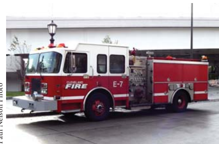
2002 Luverne 1500/500 pumper built on a Spartan Metro Star FF cab and chassis
