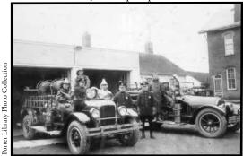
Chemical engine (left) and pumping engine (right) Fire station built onto end of police station/jail
