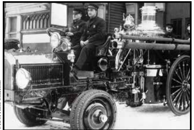
Engine 14 1916 ALF 750gpm double piston steamer
